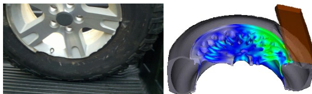
Left: photo of rim damage after curb strike. Right: results of a simulated curb strike.
